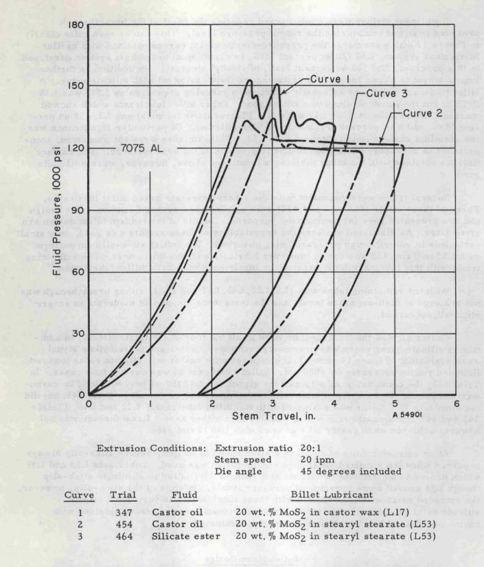
FIGURE 14. EFFECT OF FLUID AND BILLET LUBRICANT ON PRESSURE-DISPLACEMENT CURVES OBTAINED IN THE HYDROSTATIC EXTRUSION OF 7075-0 ALUMINUM AT A RATIO OF 20:1
